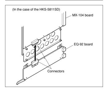
3. Secure the EQ board with the eight screws removed in step 1.
